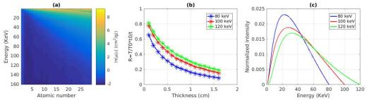
Figure 1: (a) map of  $\mu(E)$  for atomic element number from 1 to 29 and for the acceleration tension from 0 to 160 keV, (b) curves of ratio T/T0 normalized by t0/t related to the phantom thickness for acceleration tension of 80, 100 and 120 keV, (c) the corresponding estimation of X ray spectrums obtained with each curve of (b).
